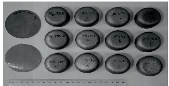
Fig. 7. Photograph of drawpieces made of AZ31 magnesium alloy sheets 2.0mm thick after cupping test by a cylindrical punch of 40 mm diameter
