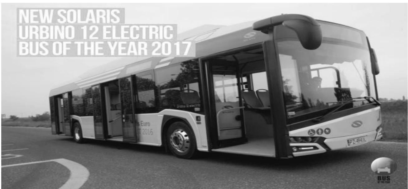
Fig. 1.1. Bus of the year 2017 -Solaris Urbino 12 Electric. It has got two systems installed – the depot charging and the opportunity charging [1]
