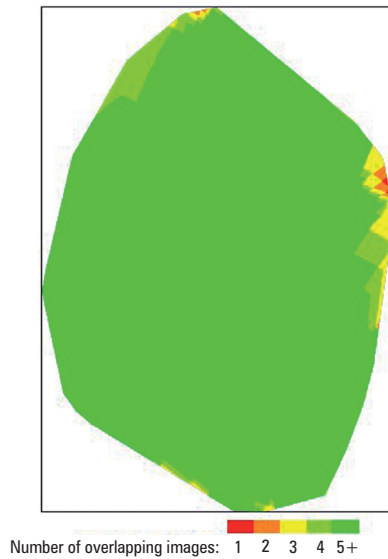
Fig. 6. Number of overlapping images computed for each pixel of the orthomosaic
