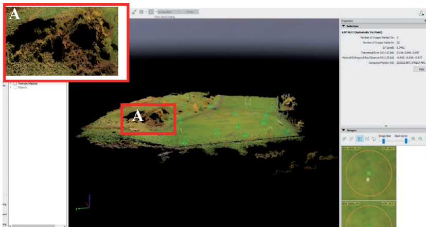
Fig. 8. Point cloud generated showing the 3D reconstruction of trees
