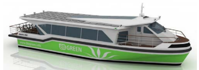
Figure 14. “BB Green Airi El” with PV panels array on its roof (source: Transport Research and Innovation Monitoring and Information System)
