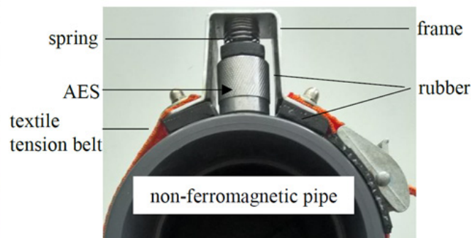
Fig. 4. AES fixing with a textile tension belt, type H3.1 [5]
