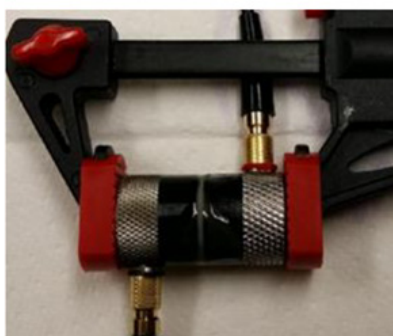
Fig. 3. Fixing two AES “face-to-face” (F2F) with a clamp, type H.2.2 [4]
