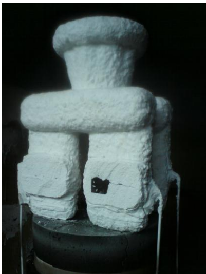
Fig. 3. The ceramic shell mould with thermocouples, after pouring with IN-713C superalloy
