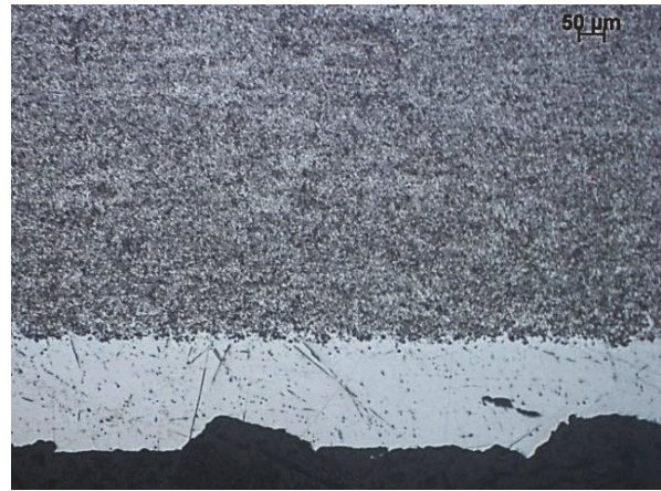
Fig. 9. Structure of the AlSiCu3 PM material anodised surface layer with 15% Al 2 O 3 powder addition.
