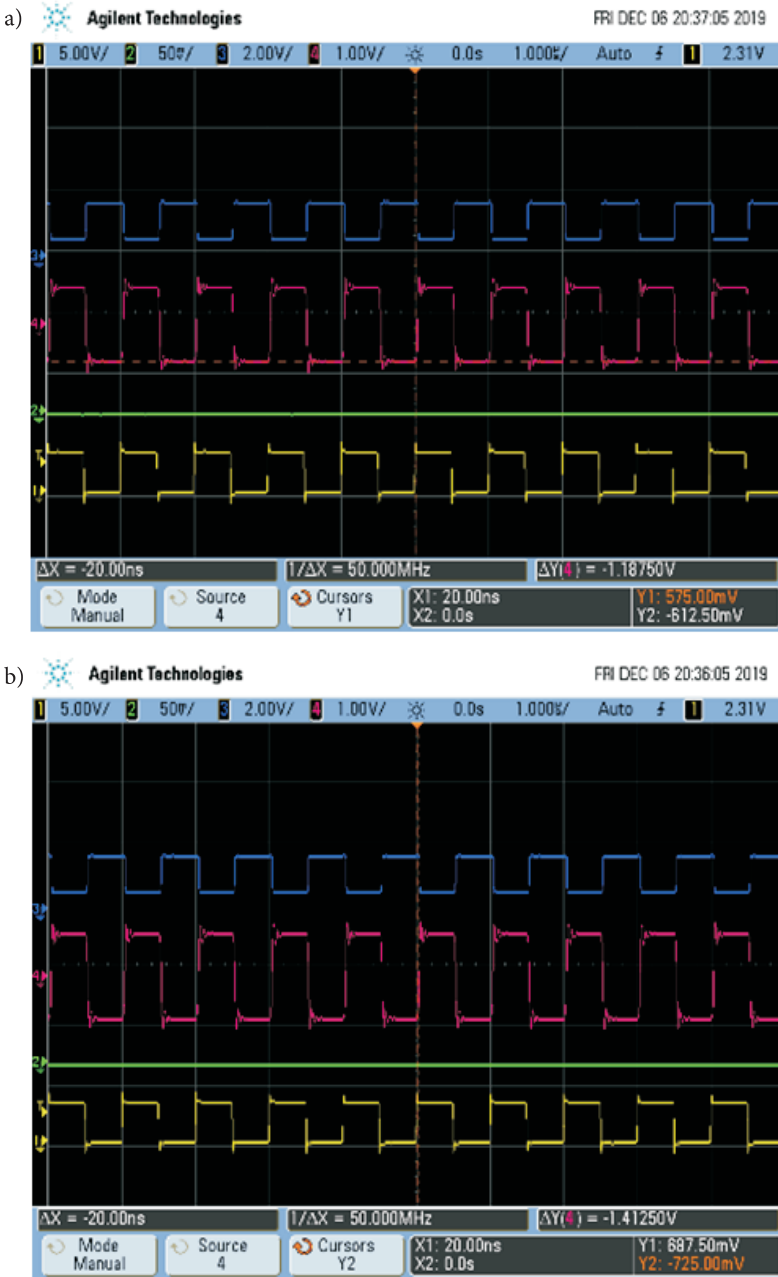
Fig. 6. Oscillograms from the connector signals in two positions: a) most unfavourable, b) most favourable, yellow — signal triggering the connector’s transmitting system, red — signal at the stage II amplifier output, blue — signal at the comparator output, and green — signal at the stage II amplifier output of the opposite detection area
