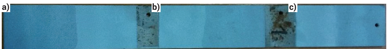
Fig. 4. The appearance of the samples with a thickness of 0.5 mm (a), 0.75 mm (b) and 1 mm (c) after testing at elevated humidity
