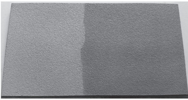
Fig. 3. Appearance of the sample with a coating thickness of 1 mm after testing at cyclically varying temperature
