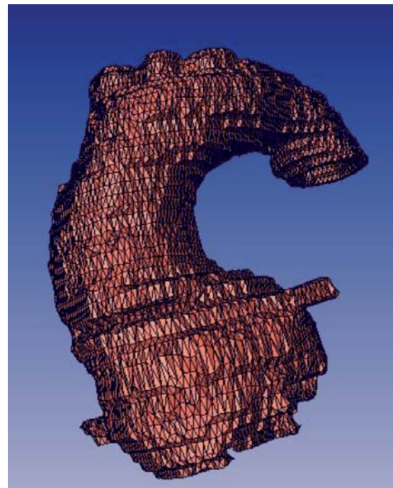
Figure 1. Early slice-stacked CAD model of the ascending aorta
