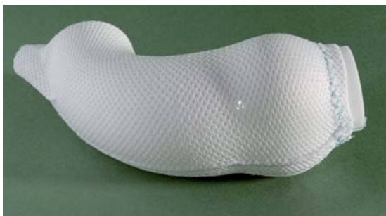
Figure 5. ExoVasc® textile implant on manufacturing former
