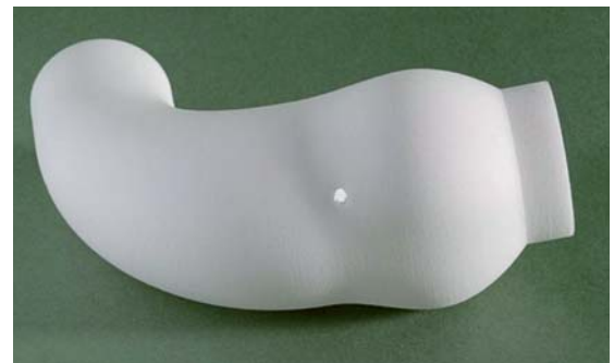
Figure 3. SLS aortic former for PEARS manufacture
