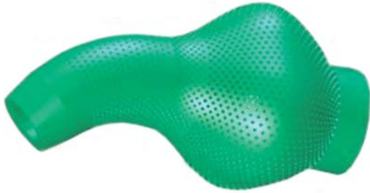
Figure 4. Porous former for vacuum formation of fibre-based implant.
