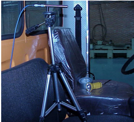
Fig. 8. Position of the microphone inside the cabin.
