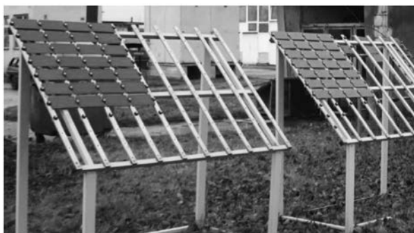
Fig. 1. Samples of coatings located on racks in climatic station
