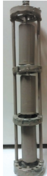
Fig. 8. Schematic of sandstone cores placed in a holder inside a PVC tube
