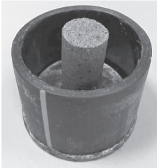
Fig. 12. Core sample to be filled with cement slurry
