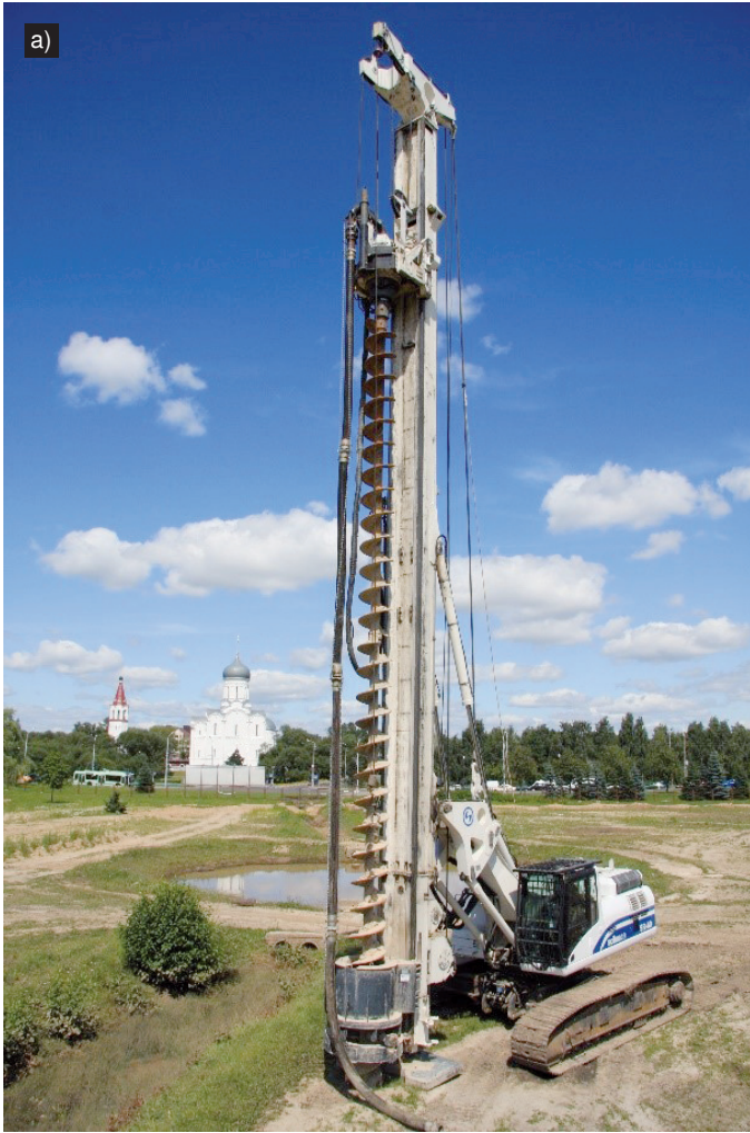
Figure 14. Equipment for piling CFA: a – drilling rig with a solid hollow auger, b – drilling rig for excavating of wells; c – lifting of the auger and installation with the vibro hammer after that installation the reinforcement cage
