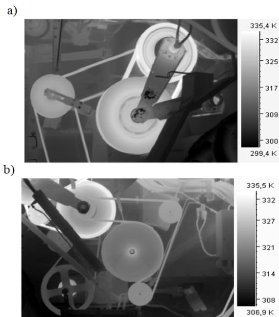
Fig. 2. Thermographs of belt transmissions: a - Massey Ferguson 7256, b - Massey Ferguson 36
