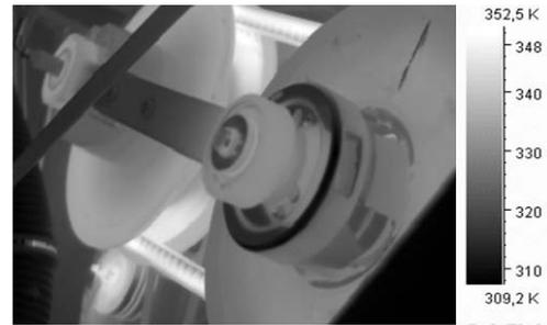
Fig. 5. Thermograph of a drive belt transmission in thresher harvesters Claas Lexion 760
