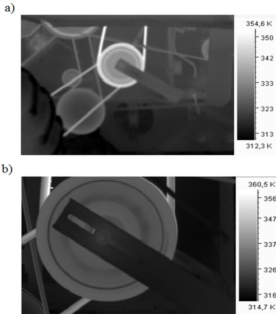
Fig. 1. Thermographs of a Bizon Z054 grain harvester: a – view from the right, b – belt pulley of variable-speed transmission of the propelling system
