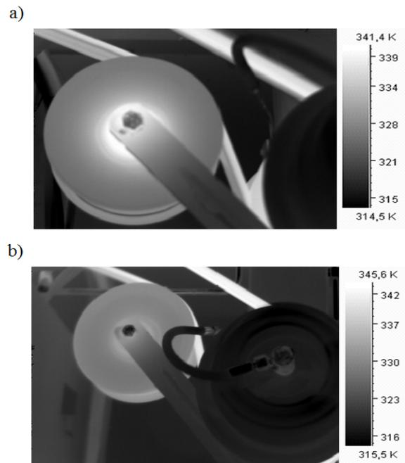
Fig. 3. Thermographs of tensioning rolls: a – New Holland TC 5080 ( $T_{\max} = 341.4$  K, representing the temperature of the central section of the roll), b – New Holland TC 5080 ( $T_{\max} = 345.6$  K, representing the temperature of the v-belt)
