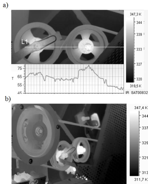
Fig. 4. Thermographs of tensioner pulleys, selected transmission in John Deere 1450: a – perpendicular position of the camera, b – camera positioned at an angle to the object,  $L_1$  – line of reference for determining the temperature characteristics T
