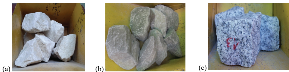
Fig. 2. Examples of feed specimens from mines in Poland with average dimension of 90 mm used in the tests: (a) limestone "Morawica", (b) sandstone "Mucharz", (c) granite "Strzegom"
