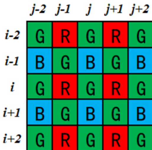
Figure 6. Bayer array of the high-speed camera, where R means red, G means green and B means blue
