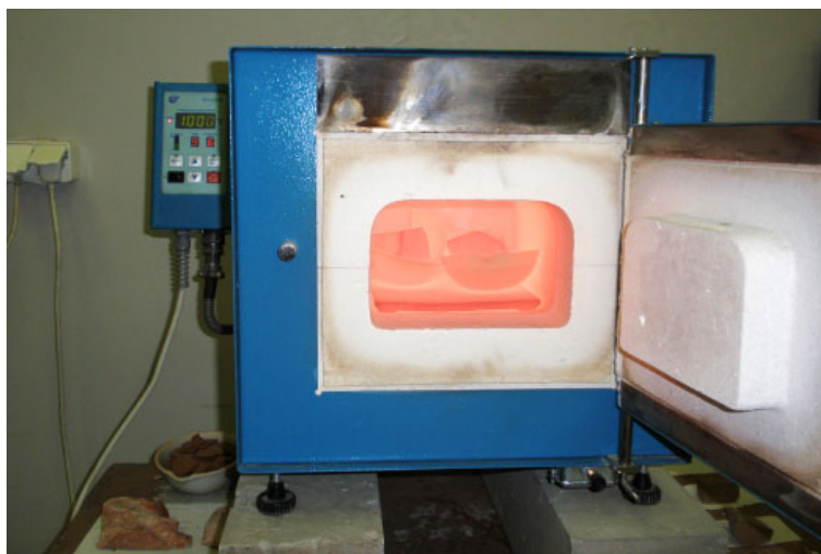
Fig. 1. Muffle kiln SM 2000 with a microchip regulator together with rock samples
