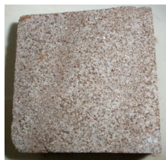
Fig. 5. Sandstone after kilning
