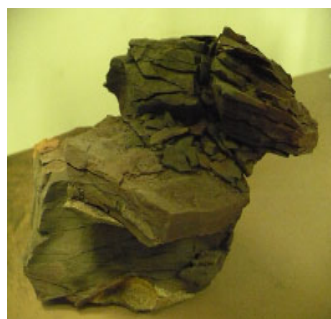
Fig. 3. Claystone after kilning
