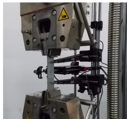
Fig. 3. The lap joints in the tensile shear testing
