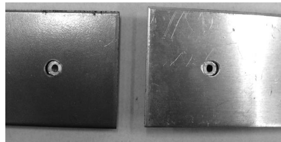
Fig. 7. COUR joints in the steel and aluminium alloy sheets after the laps separation
