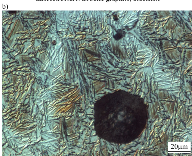
microstructure: nodular graphite, ausferrite
