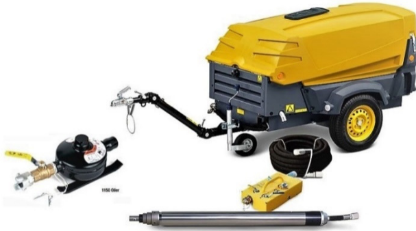
Fig. 13 Fittings for supply and control of ground rocket Source: [15, 16].
