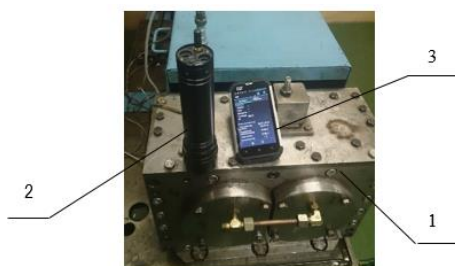
Fig. 3. Test stand: 1. investigated gear, 2. measurement device WiWiD, 3. register-analytical device (smartphone)
