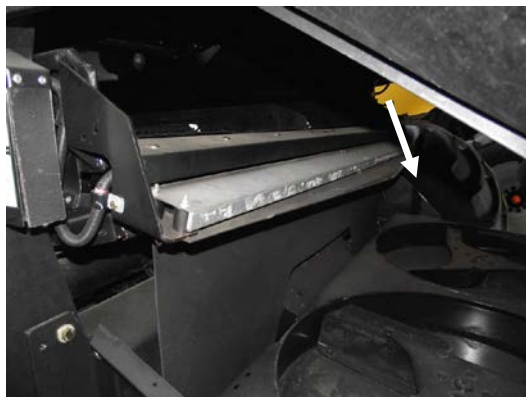
Figure 3. Sensor of losses on screens in New Holland CR 9080 (photo by author)
