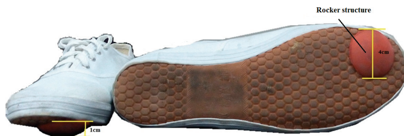
Fig. 1. The prototype of experimental shoes with rocker structure (a hemisphere 4 cm in diameter and 1 cm in height) to the outsole of hallux region (based on the rocker stiffness, Shoes-S and Shoes-H are defined)
