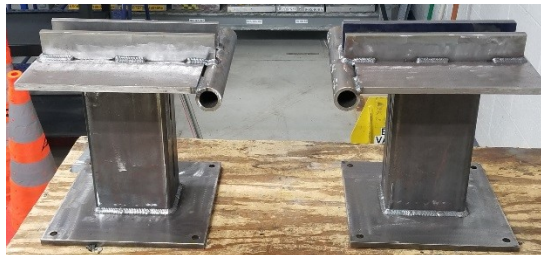
Fig. 5. Three-point bending fixture. This fixture was designed in two separate pieces to allow for various spans. The fixture allowed the samples to slide and rotate about the end rollers during loading
