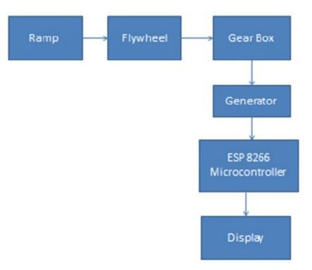
Fig. 2 Basic block diagram of energy generation
