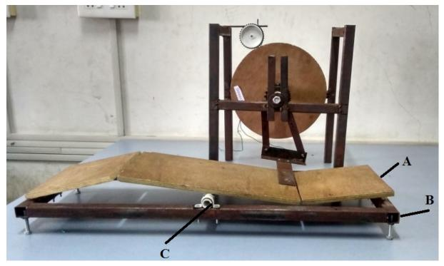
Fig. 3 Front view of the prototype model A as flat wood plate B as flat iron C as PVC pipe
