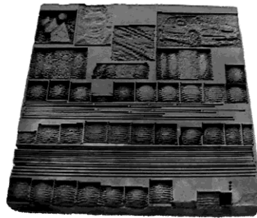
Fig. 7. Cement plate objects cut-out with high-pressure abrasive-water jet
