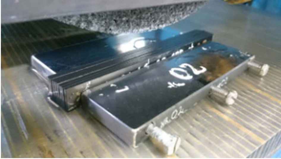
Fig. 7. Samples prepared for grinding [The Author 2016]
