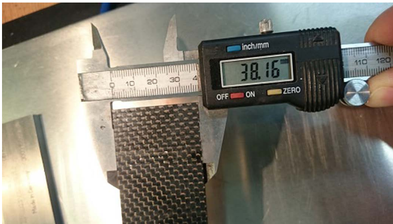
Fig. 9. Checking dimension conformity with documentation [The Author 2016]
