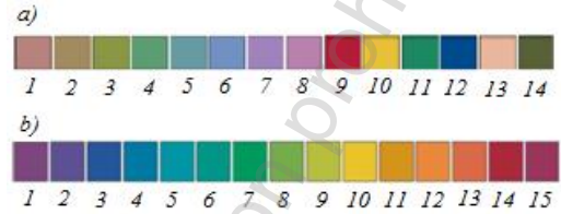
Fig. 2. Samples used in a) CRI Ra Scale, b) Color Quality Scale (CQS) (sample number increasing from left to right)
