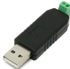
Fig.2 RS-485 – USB converter (author's photo)
