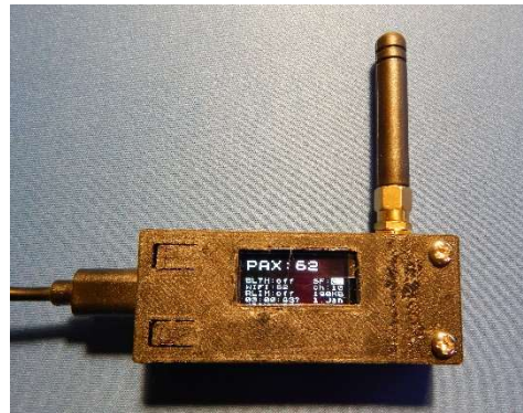
Fig.5 LoRa module (author's photo)
