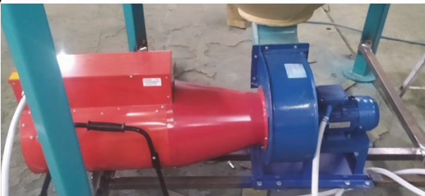
Fig. 9. General view of convective walnut dryer. a – the front view, b – the screw working body, c – system of air flow heating and injection into the drying chamber
