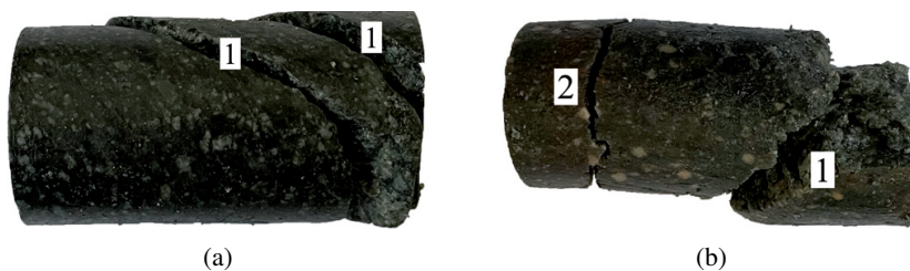
Fig. 7. Different failure characteristics of rock samples; (a) Deformation structure of high angle shear band, (b) Mixed failure structure of compression band and high angle shear band; 1 – high angle shear failure, 2 – compression band failure
