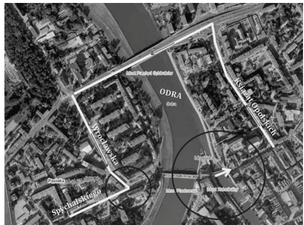
Fig. 19 Implementation of a one-way road on the Katedralny bridge will relieve the Sychalskiego street (elaboration by authors by [8]).
