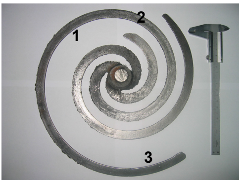
Fig. 5. Photograph of Archimedes spiral and fluidity distance L ; 1- wall thickness 1 mm, L=200 mm, 2 - wall thickness 2 mm, L=650 mm, 3- wall thickness 3 mm, L=1090 mm
