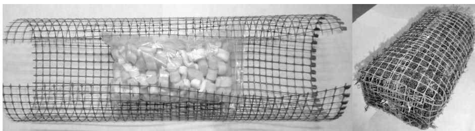
Fig. 2. Example of a moss bag, B option
