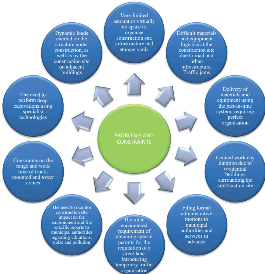
Fig. 2. Graph showing examples of constraints and problems that appear during the carrying out of construction projects in the centres of urban agglomerations. Original work based on interviews with experts.
