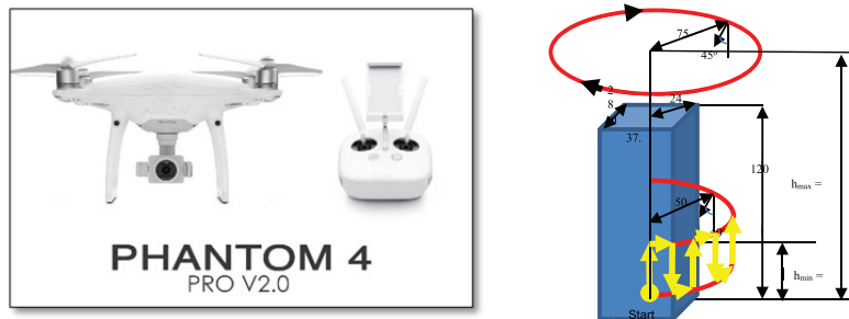
Fig. 2. Data acquisition techniques DJI Phantom 4 Pro V2.0 (a), and describe the case of taking photos of high buildings (b)
