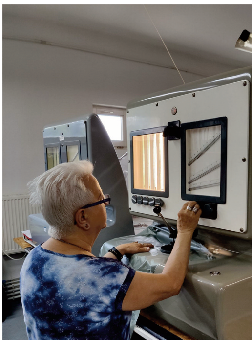
Fig. 4. Testing of the air permeability (air porosity) of the fabric of the parachute canopy [7].
