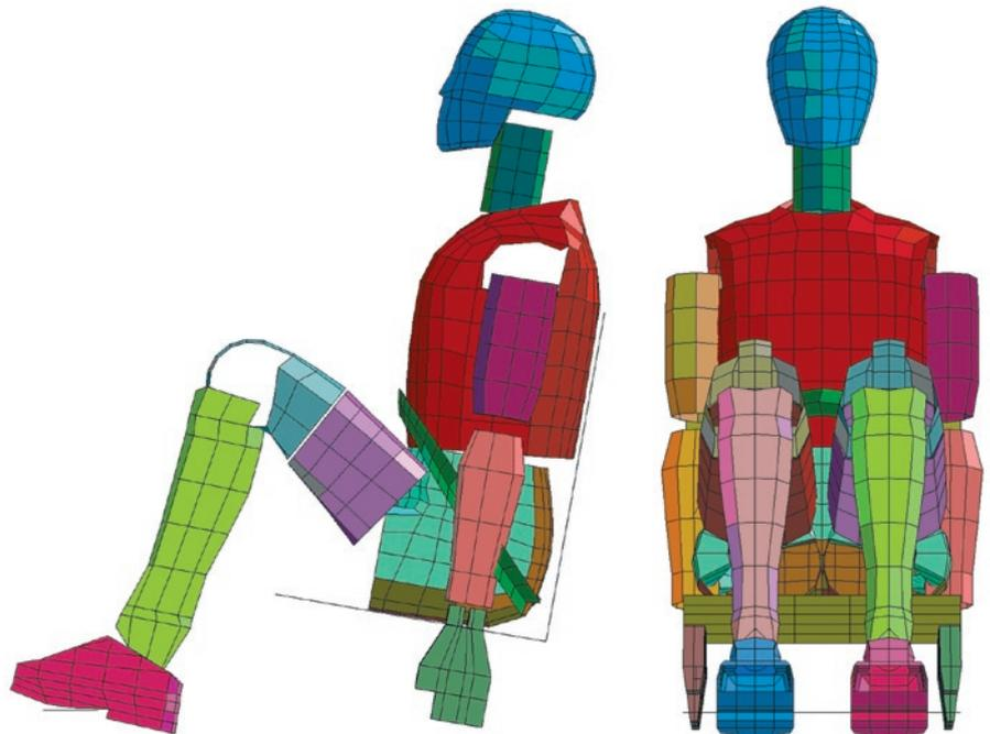
Fig. 1. Hybrid III dummy model
