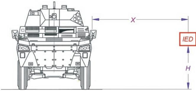
Fig. 2. Charge placement diagram relative to vehicle body
