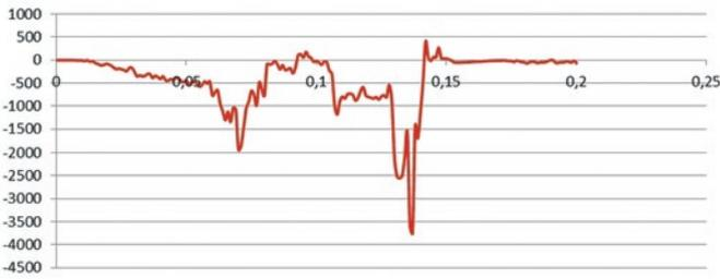
Fig. 7. Chart of longitudinal force in the spine axis Y [N] axis X [ms].
