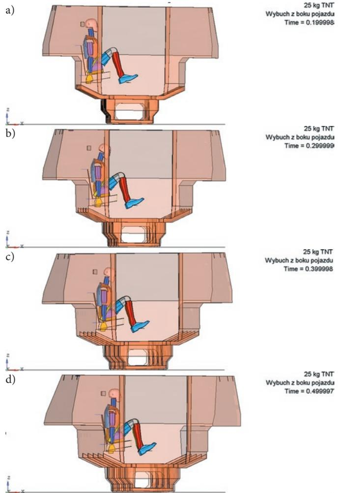
Fig. 9. The manner of vehicle body deformation and explosion's effect on a dummy in different time periods: a) 0.2 ms, b) 0.3 ms, c) 0.4 ms, d) 0.5 ms.
