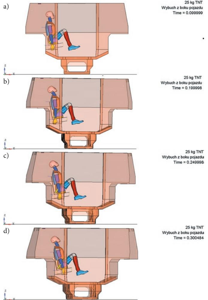
Fig. 4. The manner of vehicle body deformation and explosion's effect on a dummy in different time periods: a) 0s, b) 0.2 ms, c) 0.25 ms, d) 0.3 ms
