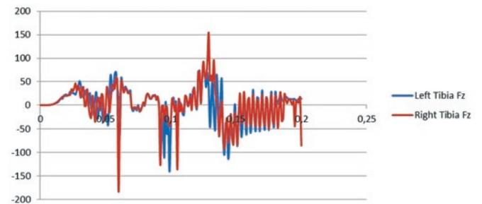
Fig. 5. Chart of longitudinal force in both tibias axis Y [N] axis X [ms]
