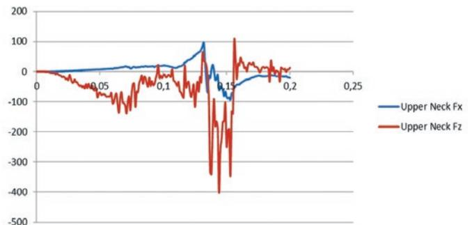
Fig. 13. Chart of longitudinal and transverse forces in the neck axis Y [N] axis X [ms]
