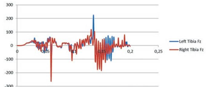
Fig. 10. Chart of longitudinal force in both tibias for the case with a headrest used axis Y [N] axis X [ms].
