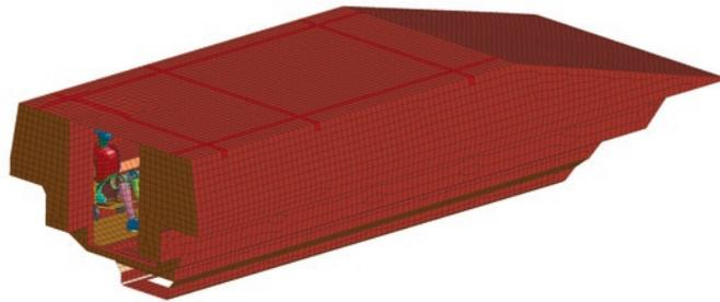
Fig. 3. Numerical vehicle model with a crew member
