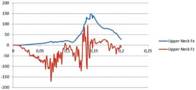
Fig. 8. Chart of longitudinal and transverse forces in the neck axis Y [N] axis X [ms]
