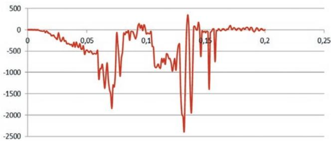
Fig. 12. Chart of longitudinal force in the spine axis Y [N] axis X [ms]
