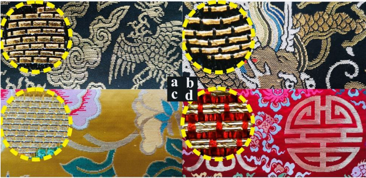
Fig. 4. (a) Zhuanghua satin woven with gilt paper lamella (gold-inclusive rate of gold foil is 99%). (b) Zhuanghua satin woven with gilt paper filé (gold-inclusive rate of gold foil is 99%). (c) Zhuanghua satin woven with alloyed paper lamella. (d) Zhuanghua satin woven with filé composed of a lamella of polyester material. Source: Nanjing Shengshijinxu Brocade Weaving Limited Company, Nanjing 210049, China
