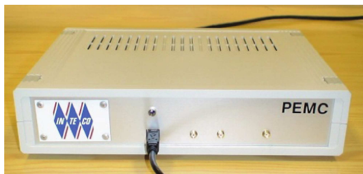
Fig. 4. General view of dedicated controller.
