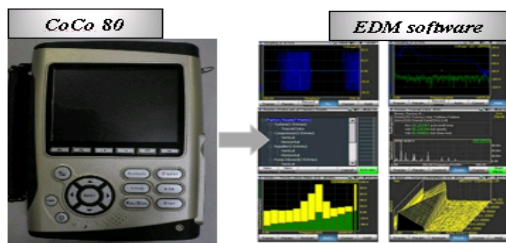
Fig. 4. The set up scheme and software outputs of the vibration measurements (Source: own study)
