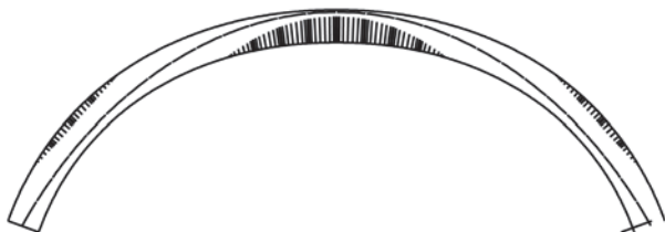
Fig. 6 The arch at 1 mm horizontal yield of the right abutment (scale factor 200)
