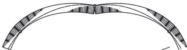
Fig. 8 The arch at 5 mm horizontal yield of the right abutment (scale factor 200). Three-hinge state
