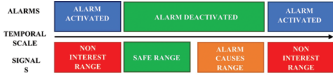
Fig. 2. Alarm and signal periods
