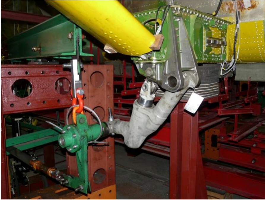
Fig. 4. PZL M28 05's wing and wing load carry-through structure fatigue test fixture. The main landing gear axle is loaded by vertical force, applied through wheel axle axis, and horizontal force, applied at the tire ground contact point (braking moment accounted for)
