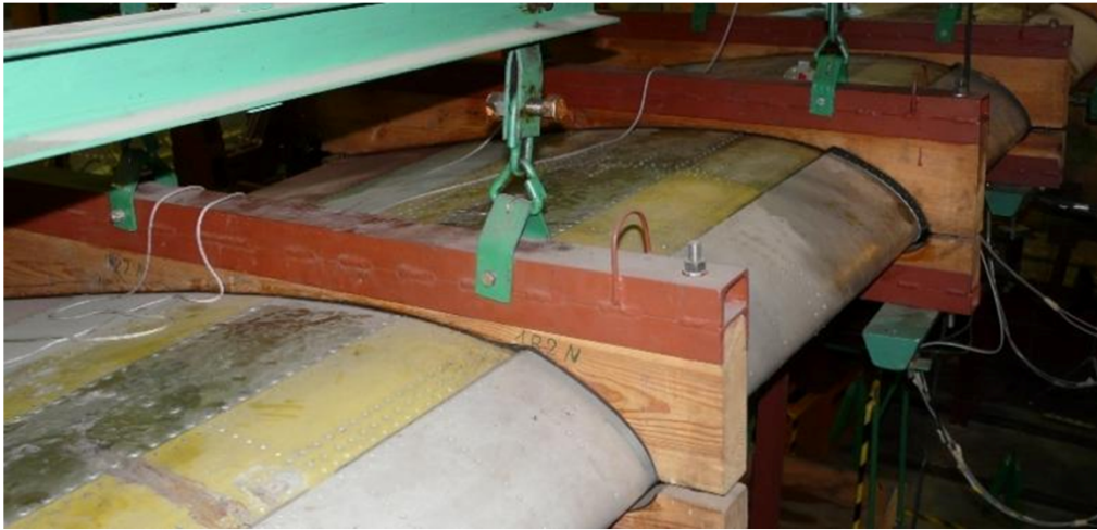
Fig. 2. PZL M28 05 wing and wing load carry-through structure fatigue test fixture. Clamps introducing loads to the wing are shown. PZL M28 wing consists of two outer wings and a centerwing. Each outer wing is loaded at 5 spanwise stations by 5 clamps, and the resultant forces are applied by two actuators. The centerwing is loaded at 5 spanwise stations: by 2 clamps at 2 stations and by glued tapes at 3 stations
