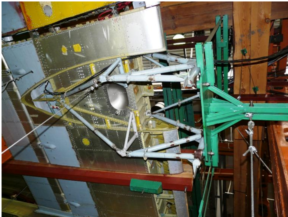
Fig. 5. PZL M28 05 wing and wing load carry-through structure fatigue test fixture. The engine frame is loaded by vertical power plant inertia force, engine torque and balancing prop thrust force
