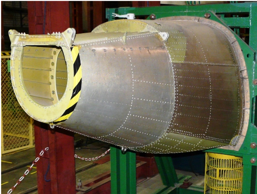
Fig. 6. PZL M28 05 empennage fatigue test fixture. The fuselage part used in test is visible on the photo (empennage is dismantled).
