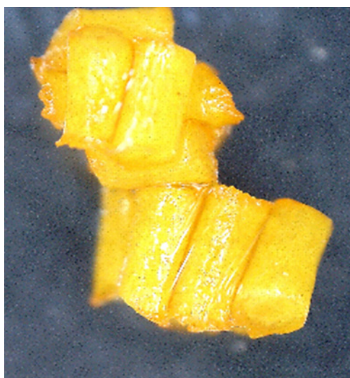
Figure 1. Glued propellant grains after P5 modification with 3 phr rosin
