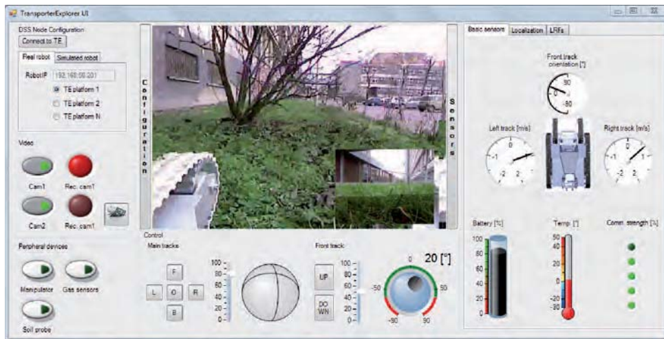
Fig. 2. Example of UI running on the operator's PC allowing to control Transporter and Explorer robots
