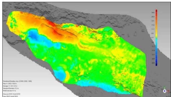
**Fig. 9.** Surface comparison of TIN models from 2010 and May 2013, top view. Green – no displacements, red – displacements of up to 34 m in the direction of the rock slide, blue – material which has been removed from the quarry
