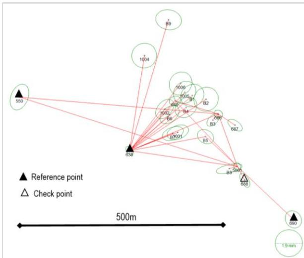
**Fig. 3.** Observational plan and standard error ellipses
