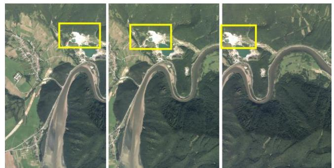
**Fig. 5.** Series of stereoscopic images taken by the UltraCam Xp large-format camera (2010) used to create DEM and an orthophotomosaic. The rock slide can be seen in the yellow boxes
