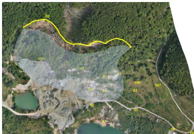
**Fig. 2.** Top view of the rock slide, its head scarps and arrangement of the observed points. The most active part of the rock slide is highlighted in white shading
