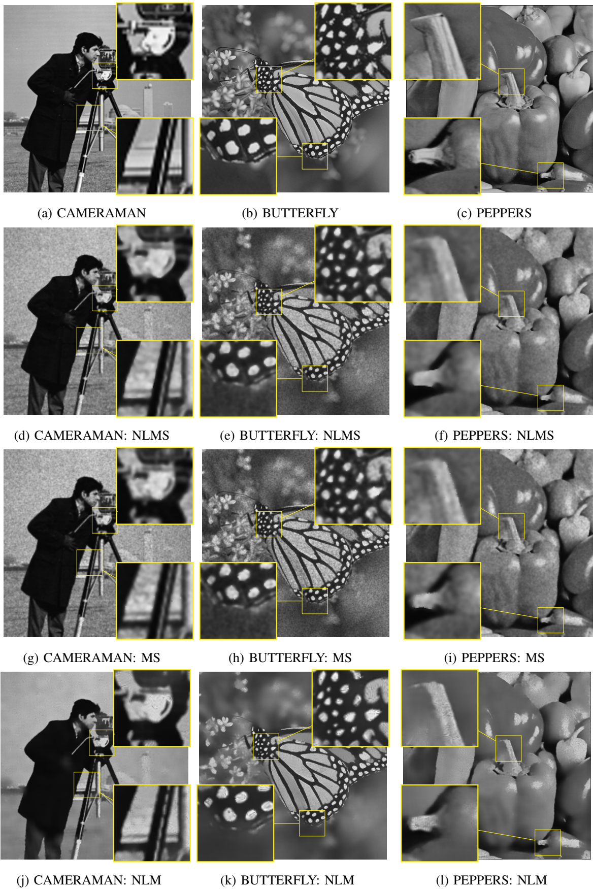
Fig. 4: Comparison of the efficiency of the proposed NLMS filter with the NLM and MS techniques using test images contaminated with multiplicative noise G_{0.3} .
