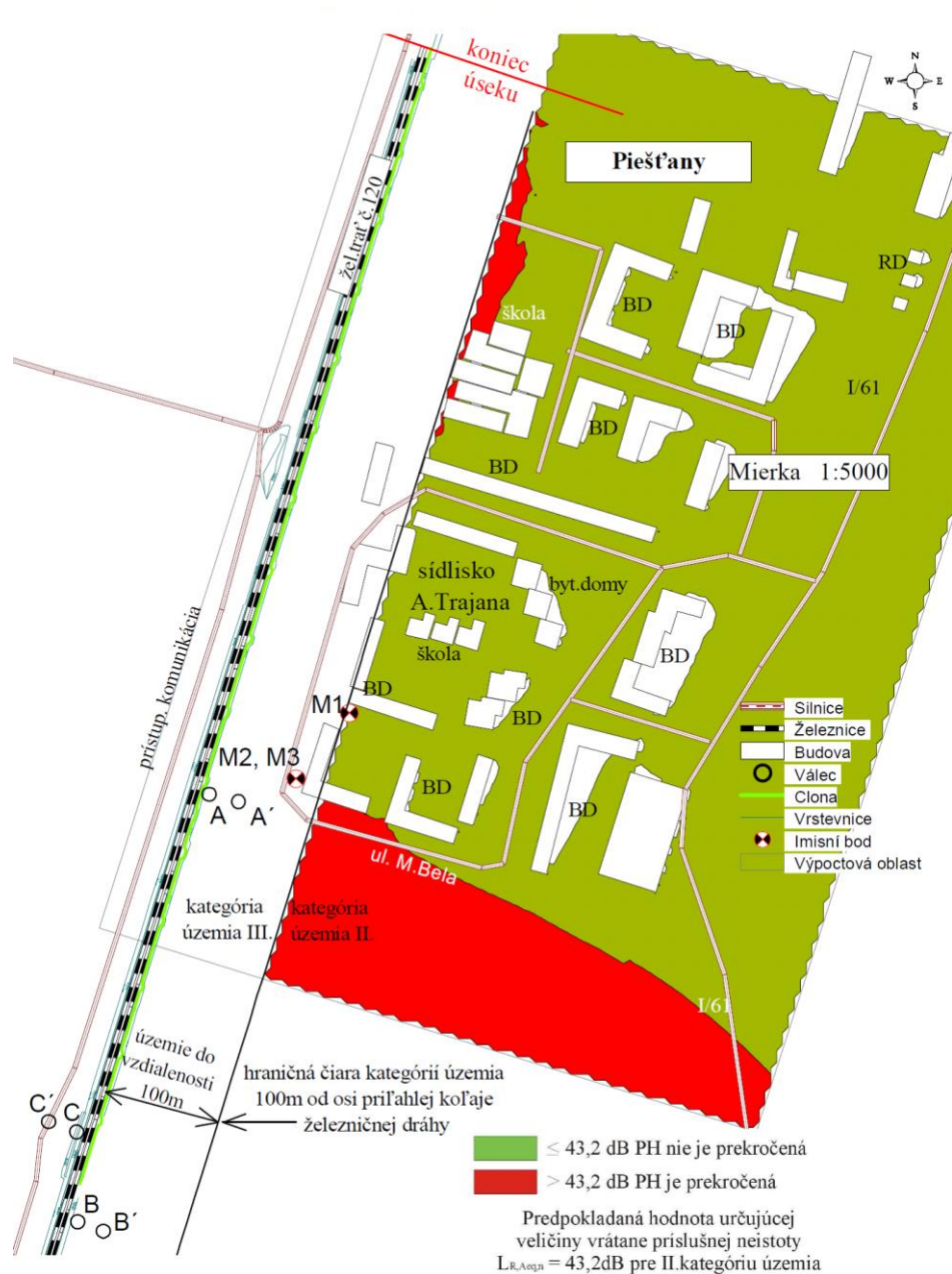
Fig. 19. Graphic output for the compliance assessment of the limit values of the noise levels in the exterior area of the town Piešťany territory in the time period 22:00-06:00 [12]
